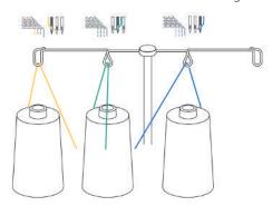
> Engage the thread in the thread pretension.
