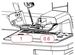
> To prevent seam puckering, reduce the differential feed to a value between 0.6 and 1.
