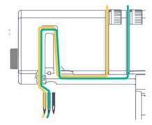
> Hook the thread into the second thread guide from left of the needle holder.
