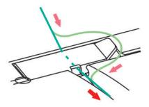
> Place the thread along the thread path between the thread tension discs.
