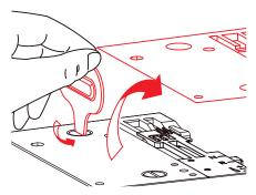
> Remove dust, fabric and thread remnants with the brush or a vacuum cleaner.
