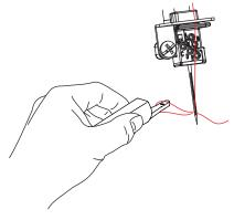
> Place the thread under the presser foot to the back left.
