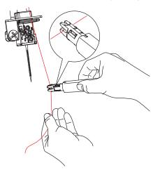
> Position the needle threader with the V-guide at the top of the needle and with little pressure slide along the needle to the eye.
