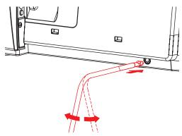
> To remove the knee lifter, pull the knee lifter out of the knee lifter connection without swinging the knee lifter sideways.
