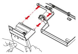
> To remove the coverstitch insert for the slide-on table, press the snap-in points downwards and pull out of the snap-in opening.
