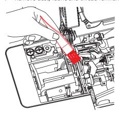
> Attach the stitch plate and screw it on.
