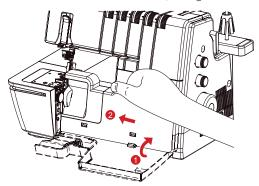
If the threader cover cannot be closed completely, the air threader connector is still switched on.
