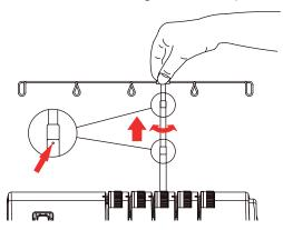
> To retract the thread guide, push the thread guide down with a little pressure.
