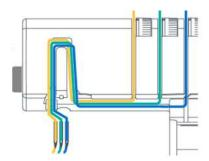
> Hook the thread into the third thread guide from left of the needle holder.
