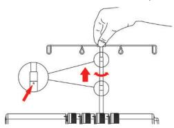
> When not in use, retract the Thread Guide with a little pressure downwards.
