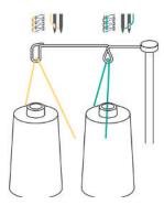
> Engage the thread in the Thread Pretension.
