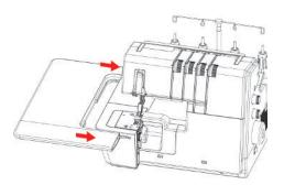
> To remove the Slide-on Table, press the Release Mechanism (1) of the Slide-on Table and pull the Slide-on Table to the left.
