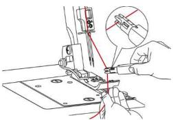
> Position the Needle Threader with the V-guide at the top of the needle and with little pressure slide along the needle to the eye.
