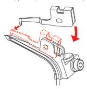
> To unhook the upper looper cover, lift the end of the upper looper cover upwards and unhook the lockin lug from the looper eye.
