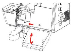
If the Threader Cover cannot be closed completely, the Air Threader Connector is still switched on.
