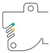
> Place the thread over the Needle Thread Take-up Lever Cover and pull it down.
