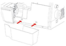
> To remove the cut-offs bin, lift the cut-offs bin out of the snap-in opening on the looper cover.
