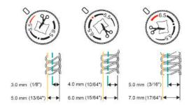
The numbers on the scale correspond with the actual Cutting Width in mm from the Left Overlock Needle «LN» to the cutting edge. The Cutting Width is used to determine the stitch width. The set Cutting Width is indicated at the Cutting Width Dial. (see page 48)
