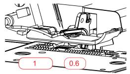
> To prevent seam puckering, reduce the differential feed to a value between 0.6 and 1.
