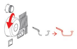
> Feed the thread through the Thread Guide.
