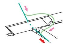
> Place the thread along the Threading Path between the Thread Tension Discs.
