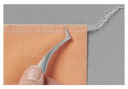
> Pull the needle thread out of the seam.
