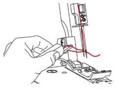
> Place the thread under the presser foot to the back left.
