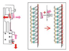
> To minimize the loops of the looper thread at the fabric edge, turn the mtc micro thread control in «-» direction while sewing.
