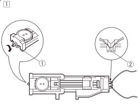
With the buttonhole foot with slide raised, hook the filler cord on the cord pin at the back of the buttonhole foot with slide.
