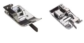
This presser foot with guide facilitates topstitching edges, hems and pleats; it is helpful when sewing on lace or ribbons and to reinforce edges. The guide lets you sew perfect seams and hems running parallel to the edge.
