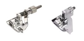
This foot is best suited to sew blind hems or to topstitch edges. The stitches only pierce the hem so that the stitch holes are hardly visible on the right side of the fabric.
