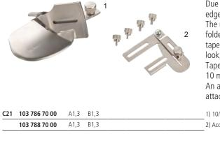
Due to the top bottom double fold binder attachment, fabric edges and necklines can be perfectly bordered with bias tape. The unfolded tape is inserted through the attached guide rail, folded over twice on the upper and lower sides of the bias tape and sewn on with a cover or chain stitch. For the perfect look, the bias tape can also be self-made.
