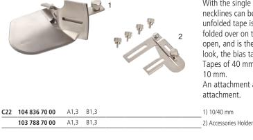
With the single fold binder attachment, fabric edges and necklines can be perfectly bordered with bias tape. The unfolded tape is inserted through the attached guide rail, folded over on the upper side while the under side remains open, and is then sewn on with a cover stitch. For the perfect look, the bias tape can also be self-made.
