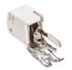
Fabrics that are difficult to work with are best sewn with the Walking Foot. It supports the fabric feed with a second feed dog on the top of the foot. The sewing project is moved in synchronization with the lower feed dog to ensure a smooth sewing process.
