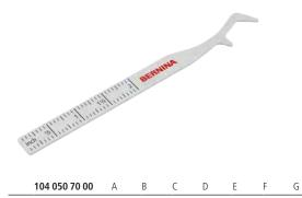
With the CS-Lock Tool, the needle threads can be pulled between foot and stitch plate easily. This eases cutting and locking the cover- and chainstitch. The scale serves as tool to measure hems, seams or mark fabrics. The scale can additionally be used to adjust the seam guide. The CS lock tool is made of soft plastic which is gentle on thread and fabric.
